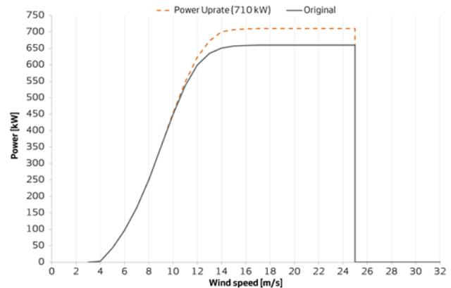
Figure 1 Power curve for Power Uprate on the Vestas V47
