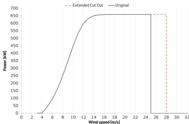
**Figure 2** Power curve for Extended Cut Out on the Vestas V47
